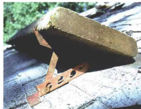
Roofbracket. On a steep roof, these brackets provide stable workstations. They are nailed through the roofing into rafters, and a plank is nailed to the brackets through holes at the front of the bracket. Because of the teardrop shape of their nail slots, roof brackets are easily removed by tapping them upward.
